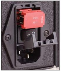
5. Close the door over the voltage selector/fuse holder. The correct voltage, that which matches the voltage of the power to be supplied to the unit, should now show through the window.
