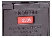
The TCV is fused at 1 Amp for 115VAC. The TCV is fused at 1 Amp for 230 VAC. The fuses are located on the sides of the voltage selector/fuse holder, as shown in the accompanying photograph.
