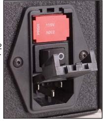
3. Turn the red voltage selector/fuse holder over so the voltage matching that of the power to be supplied has the top of the printed voltage facing upwards.
