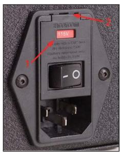
2. If the setting needs to be changed because it does not match the power to be supplied, open the access door marked as #2 in the prior image by prying outward gently with a fingernail or small screwdriver. Slide the red voltage selector/fuse holder out of the module.
