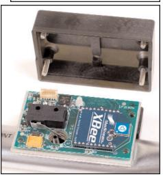
3. Gently lift the circuit board off of the mounting plate. The insulating paper (#1) is essential to preventing short circuits in the circuits. Examine the paper for tears and replace if torn or damaged. The activation stud (#2) moves when the torque wrench cycles (clicks), and moves the microswitch trigger (#3) that activates the electronics.
