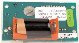
Carefully remove the tape from the holder and battery. Slide the battery out of the battery holder. Insert the new battery while maintaining the same battery holder within the battery compartment. Replace the tape, using new tape if necessary.
