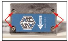
2. Gently remove the top of the transceiver housing to expose the circuit board. Gently remove the bottom of the transceiver housing from the underside of the transceiver board and mounting plate. The mounting plate is welded to the wrench.
