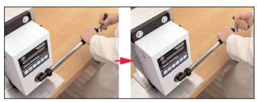
3. Install the interchangeable head on the wrench. Engage the wrench to the tester and click the wrench once or twice while noting the readings. To adjust the wrench to a higher torque setting, rotate the Torque Adjustment Key clockwise. To adjust the wrench to a lower torque setting, rotate the Torque Adjustment Key counter-clockwise. Torque adjustments should
