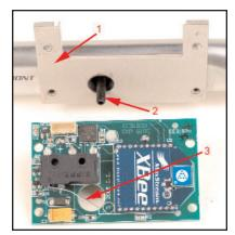
4. The battery is located on the back side of the circuit board in a battery holder. The battery is retained in place primarily by spring pressure. This retention is augmented by black electric tape as shown. Torque wrenches are sometimes subjected to shock loads that can cause a temporary disconnection of the battery, such as when the wrench is bumped against an assembly component. The tape prevents disconnection when the wrench is bumped and the force is perpendicular to the spring force.
